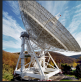
100-m Effelsberg covers the band 2.64 - 43 GHz with a precision of a few percent for monthly sampling of 60 sources
